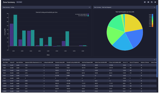
Figure 5: Dashboard showing metrics on cooling and space availability per zone
